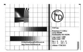
With the printing of the test card you will get your first experience with the **TOP**-*ino*. This is the internal printer test. The test card shows you the print guality and the print speed.
