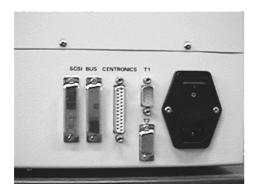
On the backside of the **TOP**-*ino* are the connectors and the power switch.
