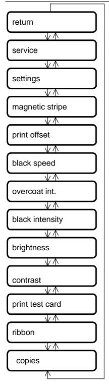
From the Off-line Mode (s. 3.2.2) to the Menu-Mode by pushing down the *print/menu* key.
